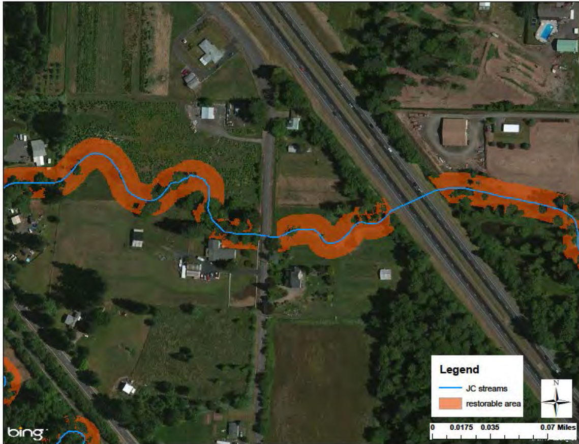
Figure 4: Example of restored conditions along streams in the Johnson Creek watershed. Area in orange corresponds to restorable area, or area within 15m of stream channel containing vegetation <4m in height.
